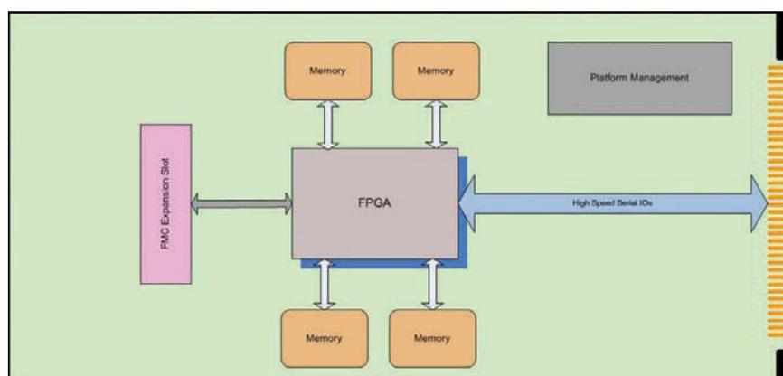
Figure 1: Typical FPGA AMC architecture
